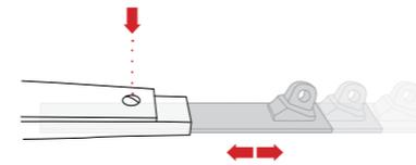
The telescopic system, besides being more immediate, is extremely precise, allowing the device to perfectly fit to the patient's physiognomy. This means significant advantages for both the comfort and the sound performance.
